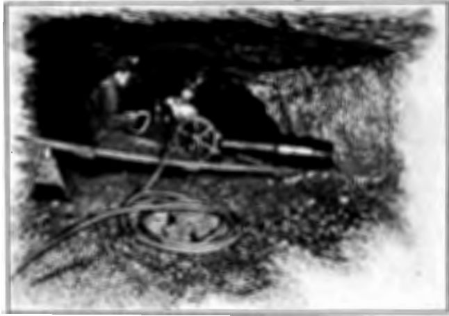
Figure 1 - Sullivan Coal Pick, showing undercut
